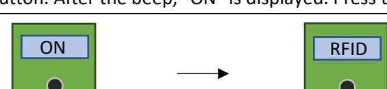
2. "RFID" appears on the display. Place a lot-specific RFID card provided with the test onto the top of the reader. This will upload the calibration data to the reader.
